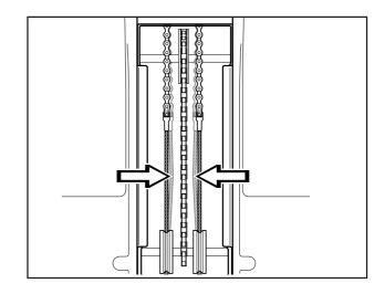
**3.** When necessary the wires can be tensioned by tightening the adjusting nuts, one on each side of the steering rim.
